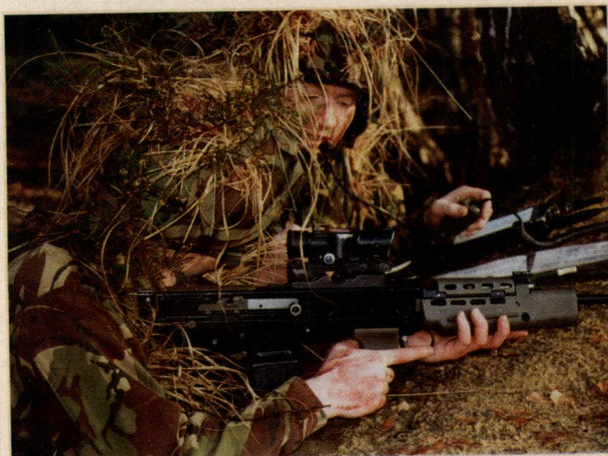
SA80 in profile. Photo shows SUSAT and cocking lever to advantage.
