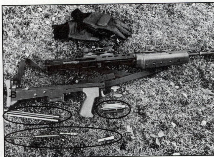
SA80 field stripped. A: shows the three components which make up the gas system. B: The recoil rod assembly. C: Bolt carrier assembly. Note this item has not been fully disassembled. Above these components the main body of the rifle is split into two parts. The lower is the trigger mechanism housing. The upper is the barrel/breech assembly.
