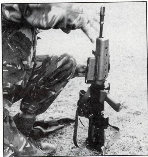
Soldier field stripping the SA80. He has opened the dust cover to gain access to the gas system.
